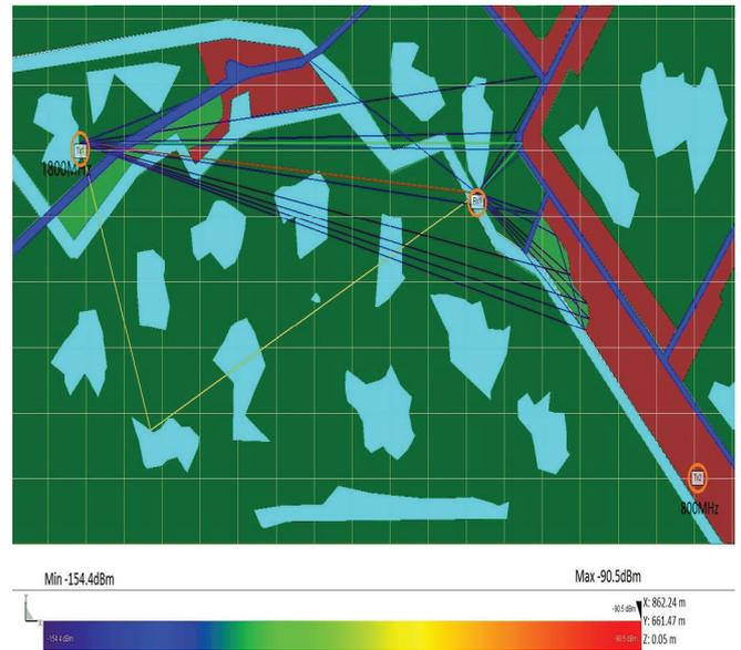
Fig. 3.3 Raytracing simulation with 50% ground water. Green – grass covered ground, blue – rain water covered ground
