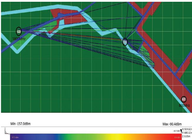
Fig. 3.2 Raytracing simulation of 1800 MHz with no ground water. This figure shows the area shown in Fig 3.1. Green – grass covered ground, blue – rain water covered ground.
