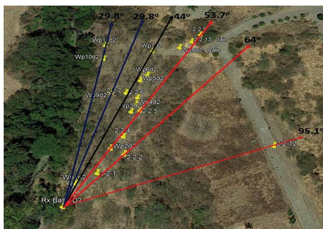
Fig. 3.7 Figure showing the radial and azimuthal measurement locations used for the RSS vs distance measurements in Colima.
