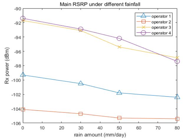
Fig. 3.5 Mean RSRP under different rainfall conditions for the four mobile network operators in the River Soar area
