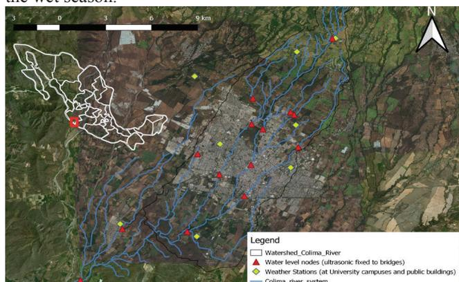
Fig. 2.2 Proposed Colima river sensor network for real time flood detection (Note white outline represents Mexico indicating position of Colima).
