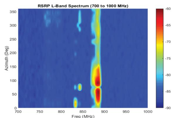
Fig. 3.6: Map of RSRP for Mobile emitters in the 700MHz to 1000MHz frequency range as a function of measurement bearing (Azimuth) in the Colima district.
