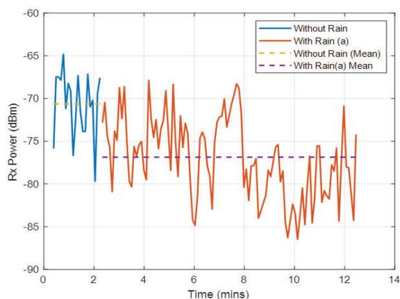
Fig 3.8 Recorded variation of received power (RSS) vs time at ‘Waypoint 2.2.13’ in Fig 3.7, with & without rainfall.
